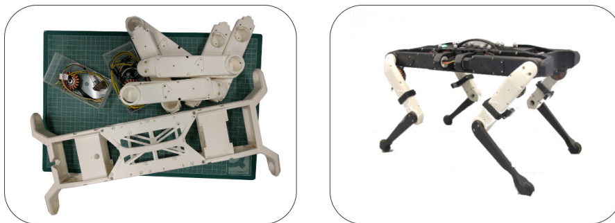
Figure 1. Solo robot. Left – 3D printed parts and motors, right – the assembled robot (source Open Dynamic Robot Initiative)
